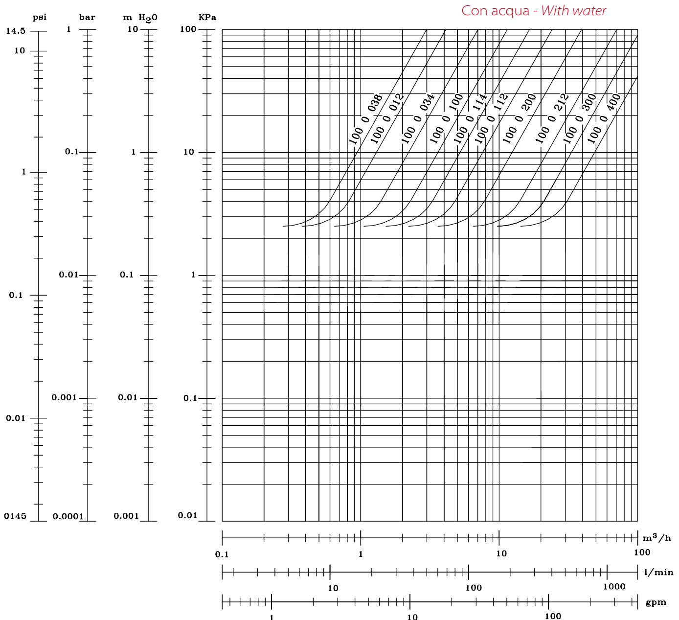
DIAGRAMMA APERTURA VALVOLA - *DIAGRAM MINIMUM PRESSURE TO GET THE VALVES OPENING*
